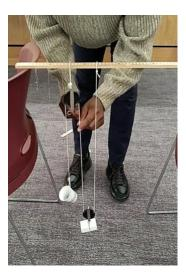
Specific Activity extension: Students explore a multiple pulley system and then re-balance out the mystery box. Students can compare the masses needed for the one pulley system to the two pulley system.
