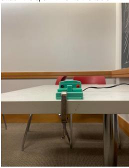
Step 2: Attach the pulley at an adjacent edge of the table to where the spark timer is.
